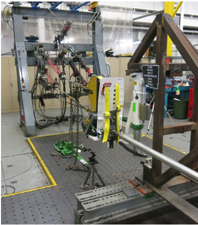
View of pull test showing rear of seat.
