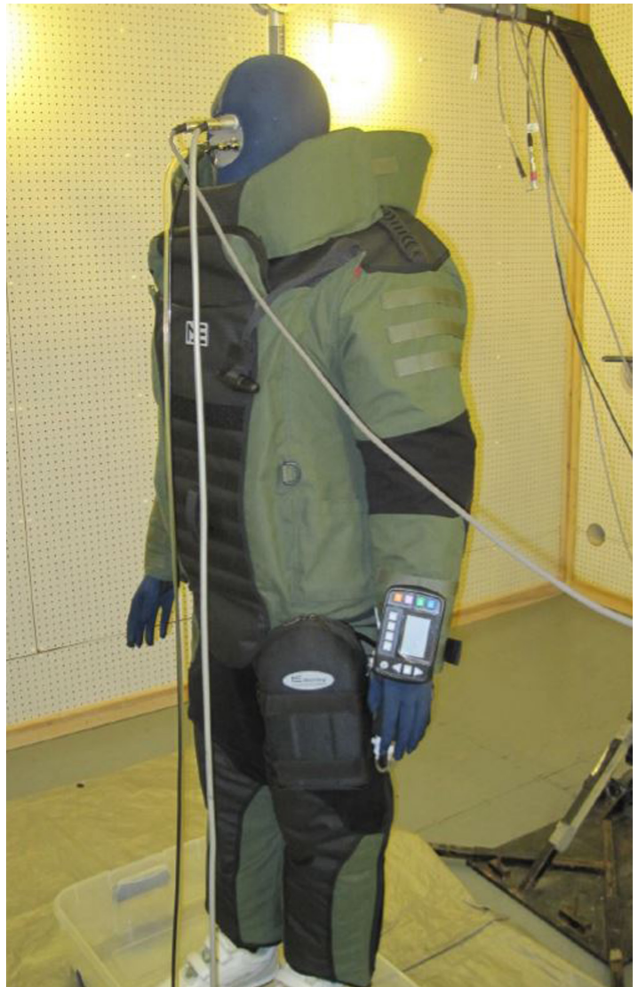
Figure 6: Personal cooling system tested in conjunction with a bomb suit against the requirements of the ASTM F2371 test methodology. Tests were conducted at the Institute of Environmental Research from Kansas State University.
