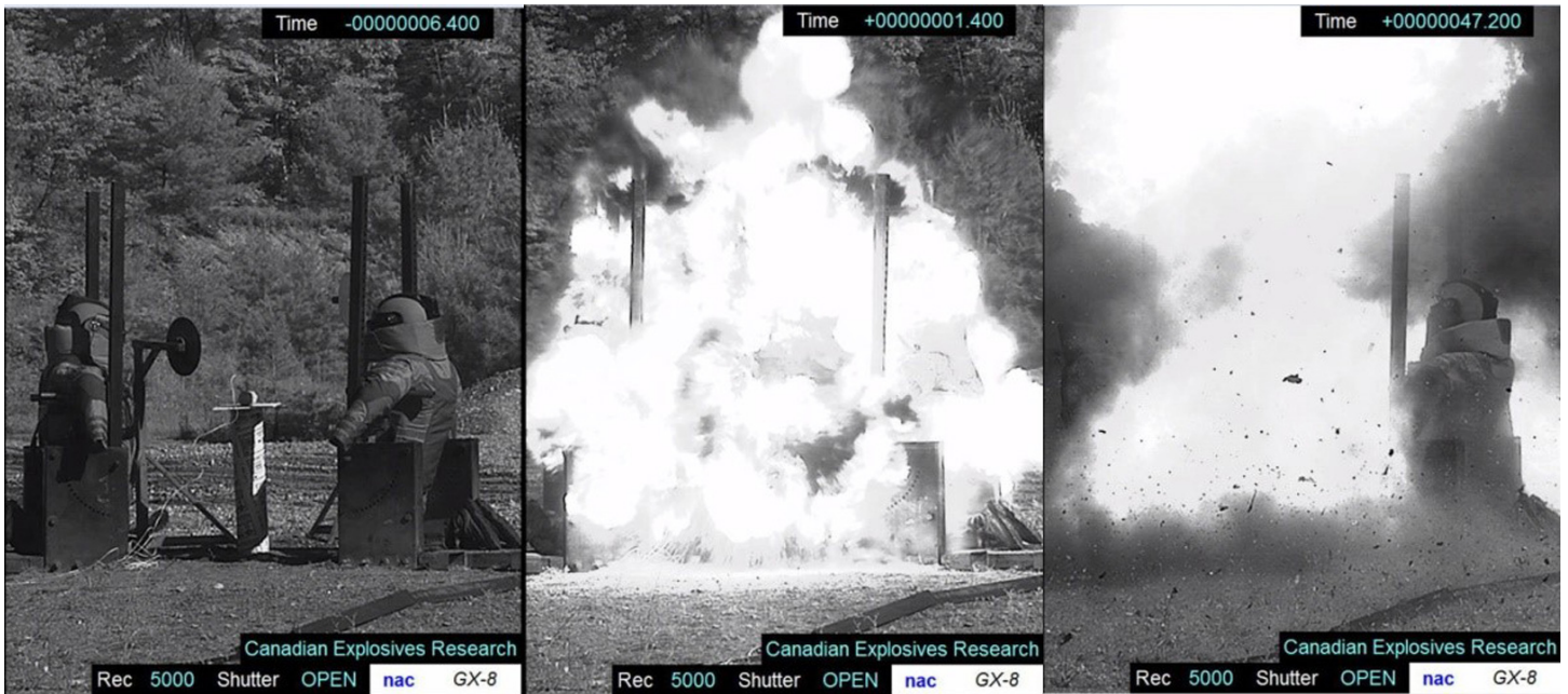
Figure 3: High speed video images of the NIJ 0117.01 blast overpressure test (0.567 kg C4 explosive, standoff 0.6 m – kneeling position). Two mannequins used for more data. Tests were conducted at the Canadian Forces Base Petawawa, under the leadership of the Canadian Explosives Research Laboratory and the supervision of Intertek auditors.
