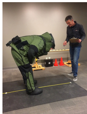
Figure 5: NIJ Dynamic FOV test – Head and Body motion with volunteer
