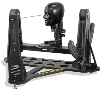
Figure 4: NIJ Static FOV apparatus – helmet fitted on a headform and tested at various angles.
